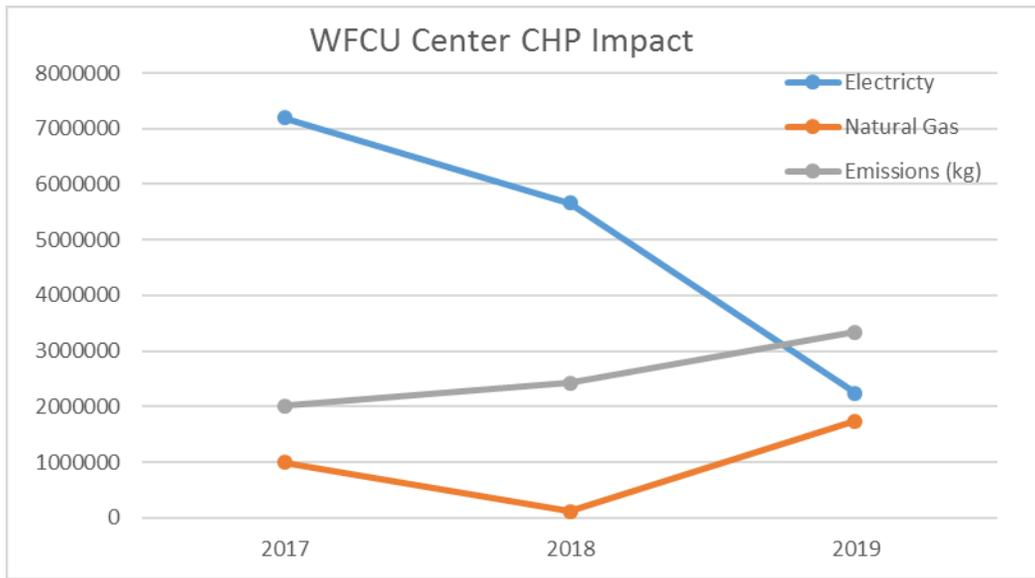
**Figure 5 – Energy Utilization and Emissions from WFCU Center**
